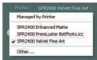
Figure 6.28 The Profile drop-down contains various options for setting the color management option to be used for the current print job.
