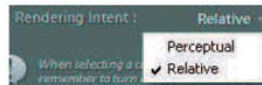
Figure 6.30 The Rendering Intent drop-down allows you to choose between the Perceptual and Relative rendering intents.
