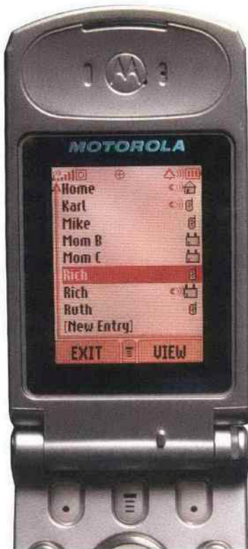
FIGURE 2-3 / This cell phone contains a linear list of entries in a phone book. At the bottom of the screen, you see a pair of softkeys—changeable labels for the hardware buttons underneath them—labeled "Exit" and "View." The lefthand button is almost always Exit for all applications (users thus can become habituated to that button). However, the righthand button changes according to what you're doing—it's always the most common action.
