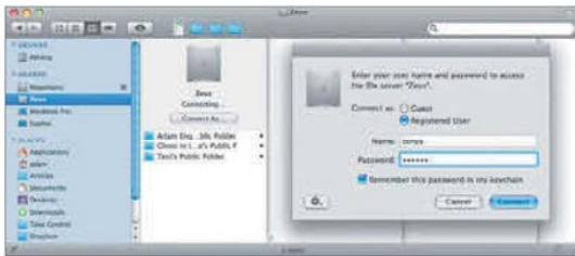
Figure 9.5 Select the host Mac in the sidebar and then click Connect As to connect to the shared Pictures folder.
