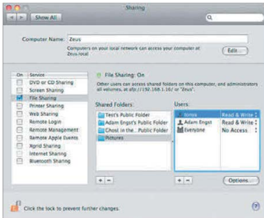
Figure 9.4 If you don't want to give everyone your user name and password to connect to your Mac, use the Sharing preferences pane to share the Pictures folder and set up login accounts for everyone.
