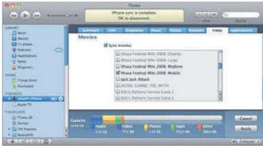
Figure 7.17 Select slideshows to sync to an iPhone or iPod under Movies in the Video tab of the device settings screen.
