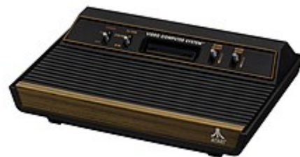
From 1980, the VCS has only four front switches and a capital-letters logotype.
