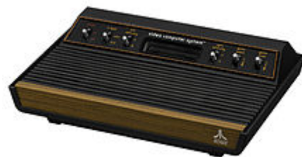
The second VCS model has lighter plastic molding and shielding, and a more angular shape, than the 1977 launch model.
