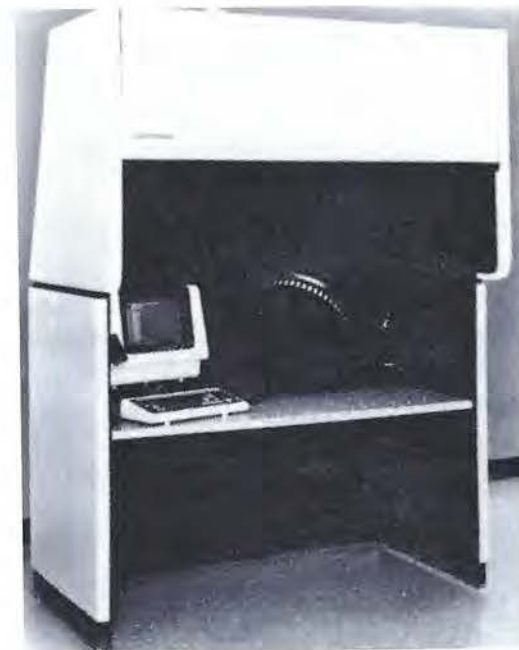
Figure 2-18 The SpaceGraph interactive graphics system displays objects in three dimensions using a vibrating, flexible mirror. (Courtesy of Genisco Computers Corporation.)
