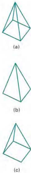
Figure 9-5 The wireframe representation of the pyramid in (a) contains no depth information to indicate whether the viewing direction is (b) downward from a position above the apex or (c) upward from a position below the base.
