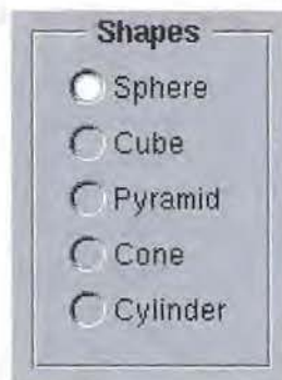
Figure 8.8 Radio-button technique for selecting from a set of mutually exclusive alternatives. (Courtesy of NeXT, Inc. © 1989 NeXT, Inc.)
