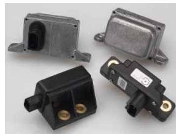
Figure 12; Packaged sensor element are packaged with electronics for automotive
