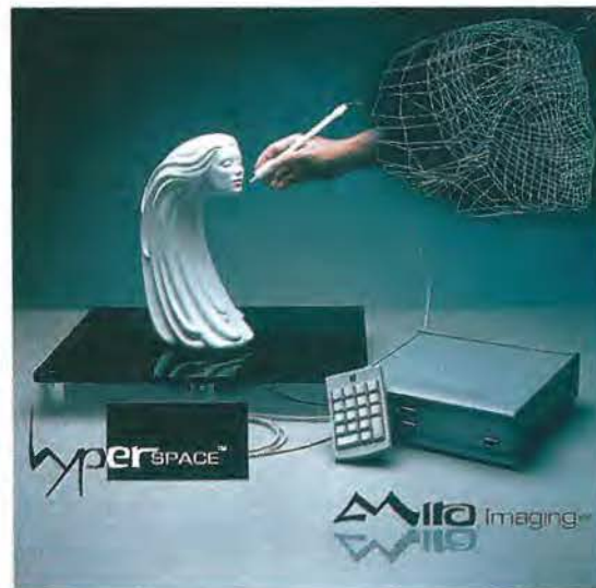
Figure 2-50 A three-dimensional digitizing system for use with Apple Macintosh computers. (Courtesy of Mira Imaging.)
