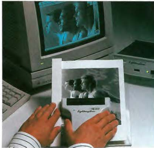
Figure 2-51 A hand-held scanner that can be used to input either text or graphics images. (Courtesy of Thunderware, Inc.)
