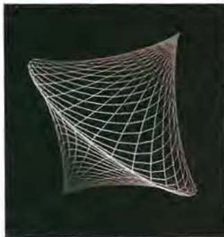
Figure 9-6 A wireframe object displayed with depth cueing, so that the intensity of lines decreases from the front to the back of the object.
