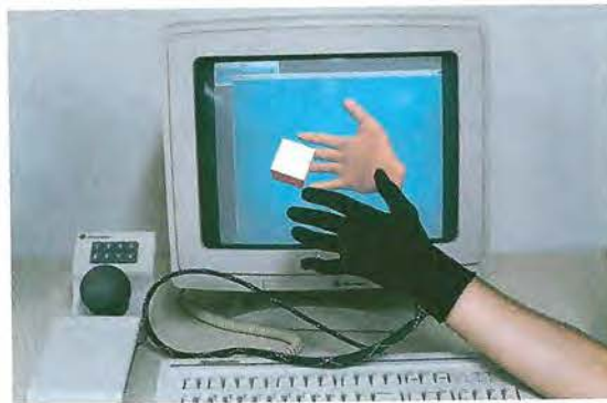
Figure 2-45 A virtual-reality scene, displayed on a two-dimensional video monitor, with input from a data glove and a spaceball. (Courtesy of The Computer Graphics Center, Darmstadt, Germany.)
