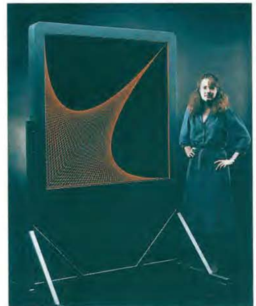
Figure 2-12 A plasma-panel display with a resolution of 2048 by 2048 and a screen diagonal of 1.5 meters. (Courtesy of Photonics Systems.)
