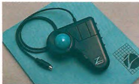
Figure 2-42 The Z mouse features three buttons, a mouse ball underneath, a thumbwheel on the side, and a trackball on top. (Courtesy of Multipoint Technology Corporation.)
