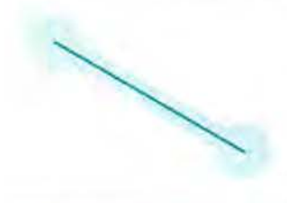
Figure 8-9 Gravity field around a line. Any selected point in the shaded area is shifted to a position on the line.
