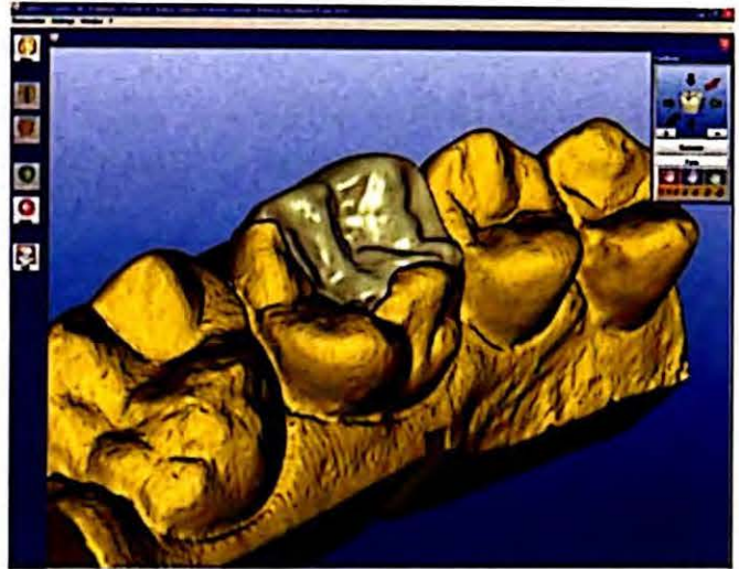
Figure 4 A screen shot of an onlay restoration proposed by the software library. User-friendly tools permit refinement of the restoration before milling.
