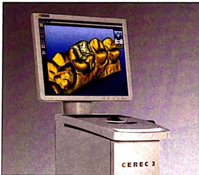
Figure 1 The CEREC 3 imaging unit. As a CAD/CAM system, the product also includes a separate, newly upgraded milling unit, the MC XL.
