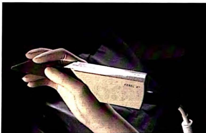
Figure 2 The CEREC 3 camera. The new software used in the system includes a camera crosshair, which makes the optical impression easier and more predictable.
