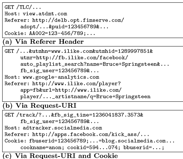
Figure 3: Leakage of OSN ID to a Third-Party From an External Application
