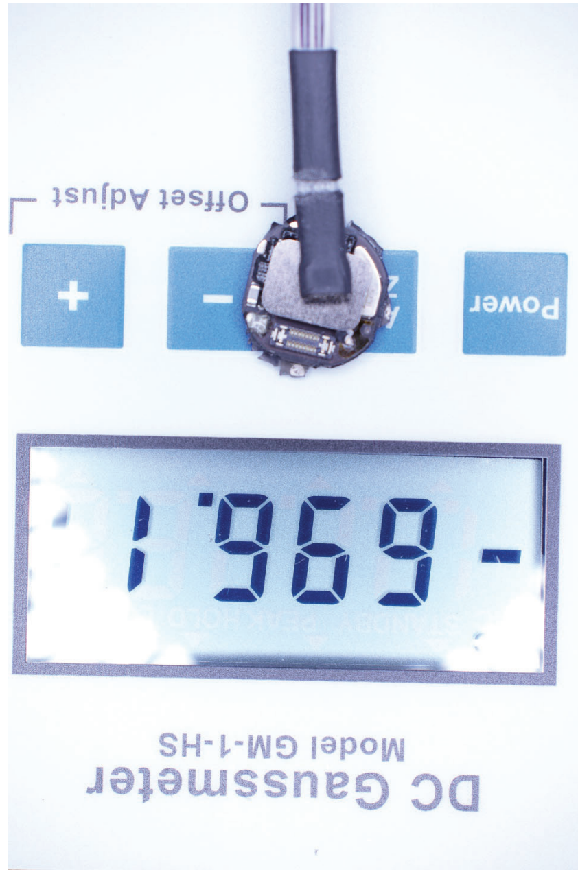
Image of the first magnet in the bottom face of the exemplary Apple Watch Series 6 from a side that faces away a wireless power transmitting apparatus. A magnetic field was measured by the the AlphaLab, Inc GM-1-HS Gaussmeter pointing inwards from the side of the first magnet that is opposite the wireless power transmitter.
