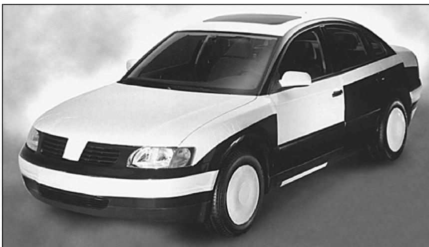
Figure 6. Temporary protection of automobile paint and other components is routinely provided by the use of polymer sheets (white areas in photograph) coated with a PSA, thus offering safe adhesion and easy removability without affecting the optical surface quality of the car even after prolonged contact time under outdoor conditions. (Courtesy of tesa AG.)
