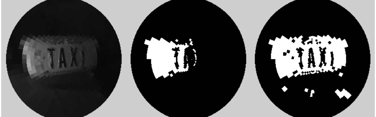
Figure 11: Example of binarization using a 2-level pyramid. The left image depicts a scene containing a license plate under uneven illumination. The middle image shows the result of applying a single global threshold. The right image shows the result of applying an adaptive local binarization procedure.
