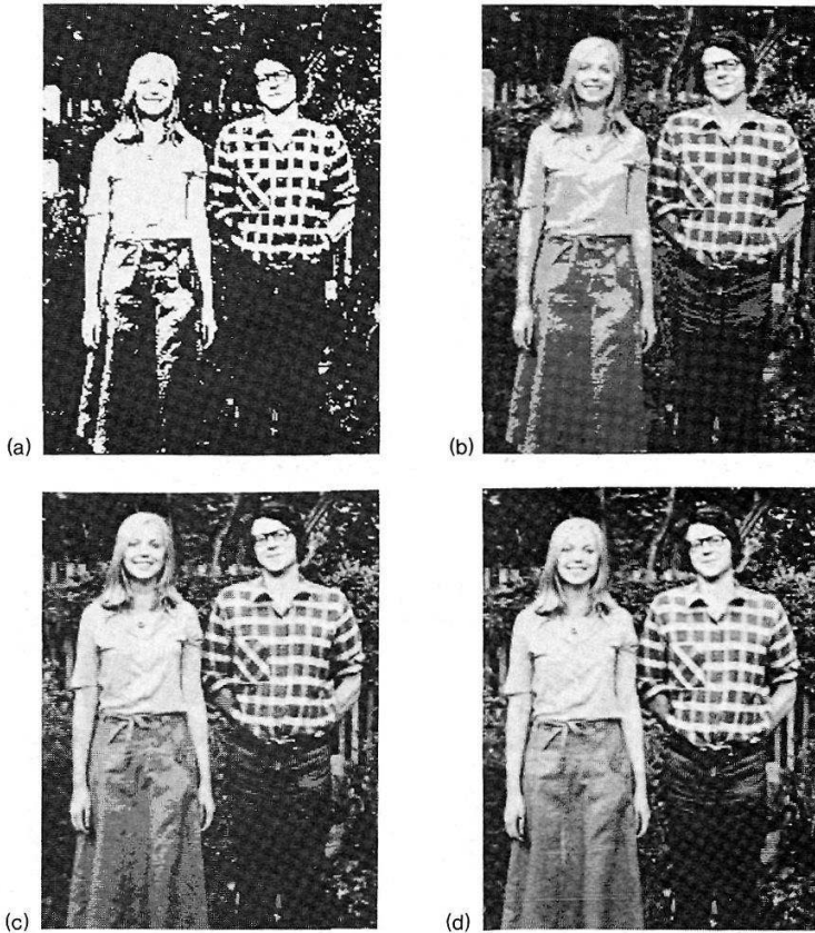
Fig. 2.10 Using different numbers of bits per sample. (a) m = 1 ; (b) m = 2 ; (c) m = 4 ; (d) m = 8 .
