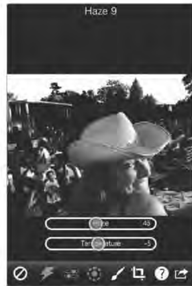
FIGURE 4-11: You can adjust a filter's parameters after a mask has been applied.
