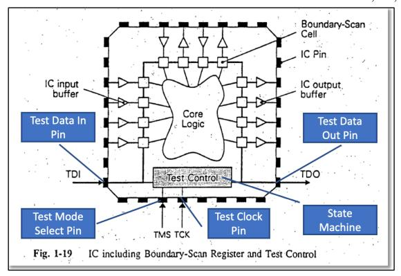
De Jong Article (Ex. 1003), 13 (annotated). As depicted in the figure, the typical boundary scan circuity is designed to test interconnects (*i.e.*, buses)<sup>1</sup> that feed information to and from a circuit using four dedicated testing pins collectively referred to as the Test Access Port to the circuit and a test controller (also called a
