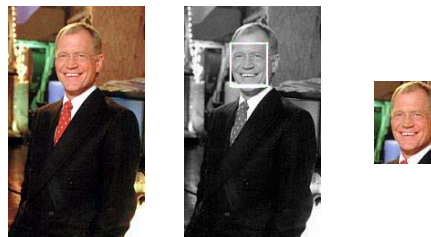
Figure 6 (left): the original image; (middle): the face detection result from CMU's online face detection [9]; (right): the cropped image based on the face detection result.
