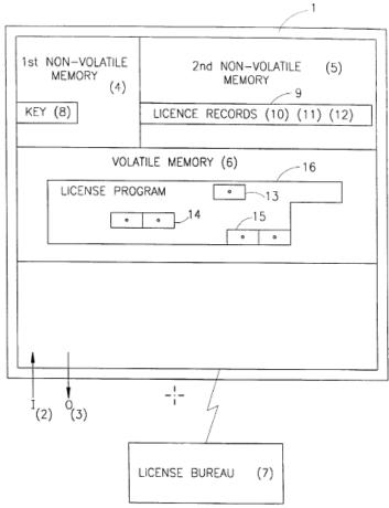
Figure 1 above shows a schematic diagram of computer processor 1 and license bureau 7. *Id.* at 5:9–19. Computer processor 1 is associated with input operations 2 and output operations 3. *Id.* Computer processor 1 contains first non-volatile memory area 4 (e.g., the ROM section of the Basic Input / Output System ("BIOS")), second non-volatile memory area 5
