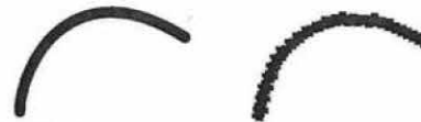
Aliasing. The lower resolution of the image on the right reveals the aliasing effect.
