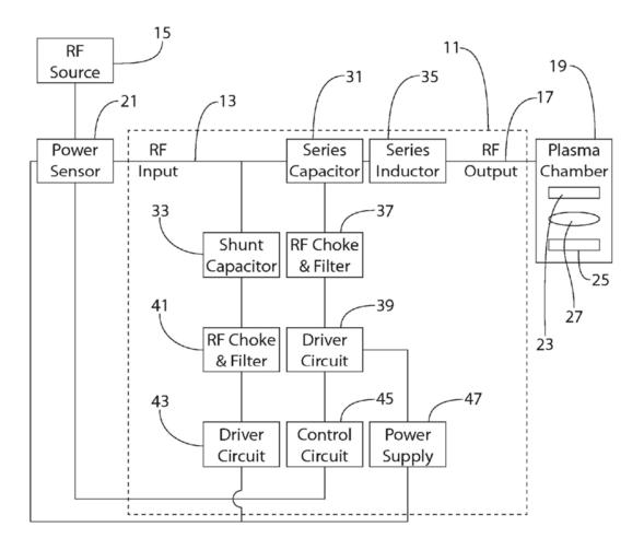
Figure 1 shows an impedance matching network using EVC incorporated into a semiconductor wafer fabrication system. *Id.* at 6:2–5.
