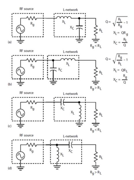
1. There are four basic L-network configurations. The network to be used depends on the relationship of the generator and load impedance values. Those in (a) and (b) are low-pass circuits, and those in (c) and (d) are high-pass versions.
