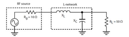
2. The RF source is a transistor amplifier with an output impedance of 10  $\Omega$  that is to be matched to 50- $\Omega$  output impedance load. The L-network with a parallel output capacitor is used.
