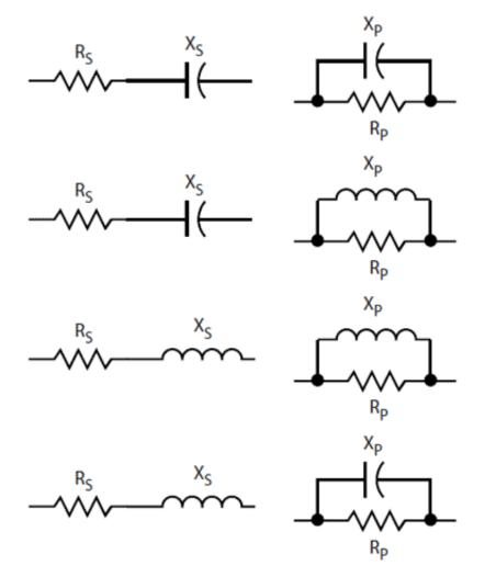
4. These are all the possible practical series and parallel RC and RL circuit equivalents. The text provides the calculations for  $R_S$ ,  $R_P$ ,  $X_S$ , and  $X_P$ .
