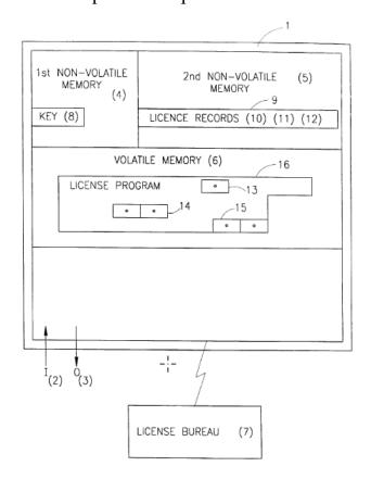
Figure 1 above shows a schematic diagram of computer processor 1 and license bureau 7. *Id.* at 5:9–19. Computer processor 1 is associated with input operations 2 and output operations 3. *Id.* Computer processor 1 contains first non-volatile memory area 4 (e.g., the ROM section of the Basic Input / Output System ("BIOS")), second non-volatile memory area 5 (e.g., the E²PROM section of the BIOS), and volatile memory area 6 (e.g., the internal RAM memory of the computer). *Id.*
