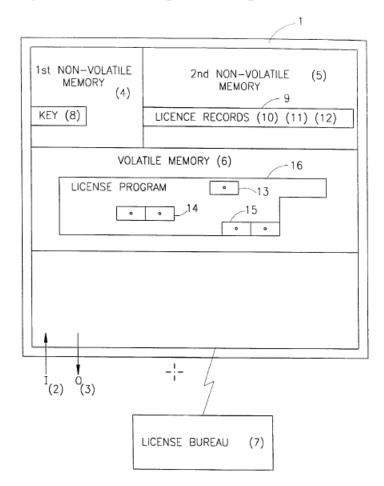
Figure 1 above shows a schematic diagram of computer processor 1 and license bureau 7. *Id.* at 5:9–19. Computer processor 1 is associated with input operations 2 and output operations 3. *Id.* Computer processor 1 contains first non-volatile memory area 4 (e.g., the ROM section of the Basic Input / Output System ("BIOS")), second non-volatile memory area 5 IPR2020-01184 Patent 6,411,941 B1
