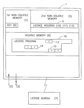
Figure 1 above shows a schematic diagram of computer processor 1 and license bureau 7. *Id.* at 5:9–16. Computer processor 1 is associated with input operations 2 and output operations 3. *Id.* Computer processor 1 contains first non-volatile memory area 4 (e.g., the ROM section of the BIOS), second non-volatile memory area 5 (e.g., the EEPROM section of the BIOS), and volatile memory area 6 (e.g., the internal random access memory ("RAM") of the computer). *Id.*
