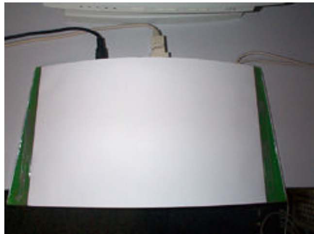
Figure 3: The MTS senses finger position, pressure, and various gestures.
