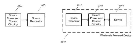
Figure 38 shows a wirelessly powered or charged device 2310 that includes or consists of device resonator 102D and device power and control circuitry 2304, along with device or devices 2308 to which either DC or AC, or both AC and DC power, is transferred. *Id.* at 58:62–59:10. The energy or
