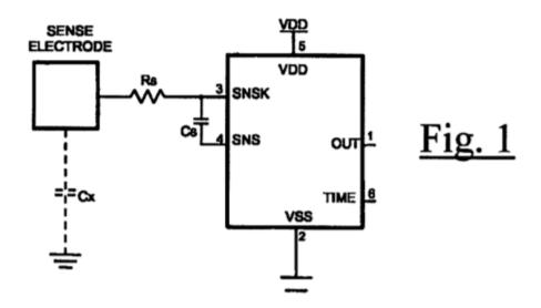
Figure 1 "schematically shows sense electrode connections for an example chip for implementing an auto-off function." Ex. 1001, 3:13–15.
