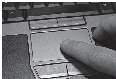
FIGURE 270. Touchpad (on a laptop computer).
