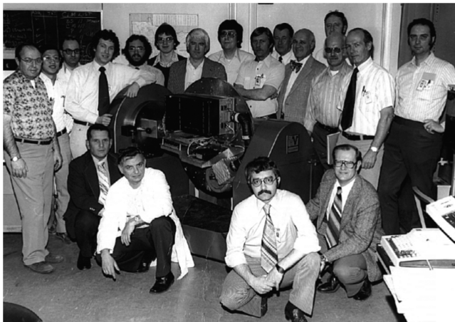
Fig. 22 Improved strapdown INS manual two-axis rotation test fixture (with Minneapolis RLG INS team).
