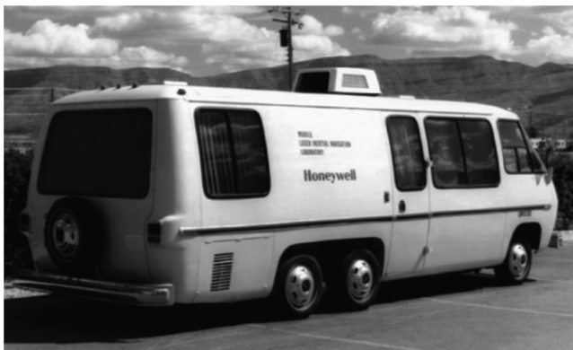
Fig. 15 LINS test van (mobile laser inertial navigation laboratory).
