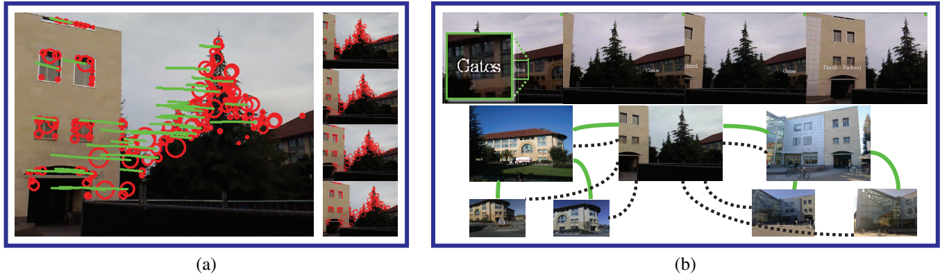
Figure 1. Our algorithm running in an outdoor environment. (a) Detected interest points and traced trajectories from a video sequence (Section 3). (b) Above: Video frames overlaid with their object labels zoomed in. Below: Matching images and their partial subgraph from the database. The solid and dashed edges indicate geometric and object ID relationships, respectively (Section 4)
