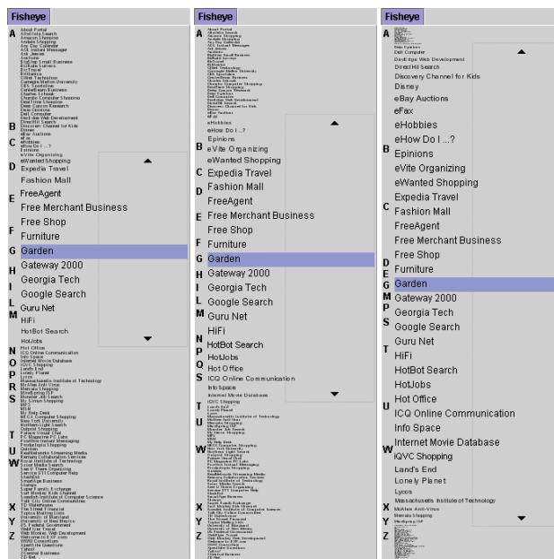
Figure 2: The same menu of 100 items displayed with varying focus lengths (7, 12, and 20). There is a fixed maximum font size.
