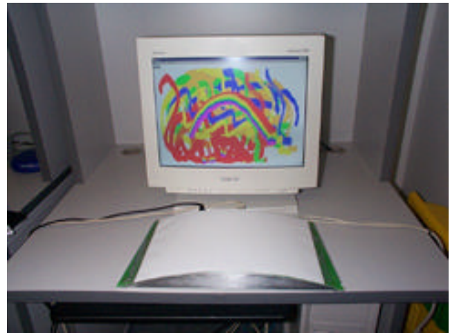
Figure 1: The Multi-Touch Surface and attached monitor. Finger strokes made on the board are transformed into paint strokes on the screen.
