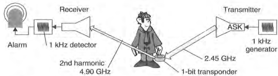
Figure 3.6 Microwave tag in the interrogation zone of a detector
