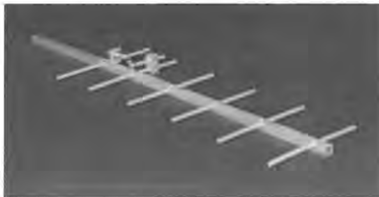
Figure 4.68 Typical design of a Yagi-Uda directional antenna (six elements), comprising a driven emitter (second transverse rod from left), a reflector (first transverse rod from left) and four directors (third to sixth transverse rods from left) (reproduced by permission of Trolleyscan, South Africa)
