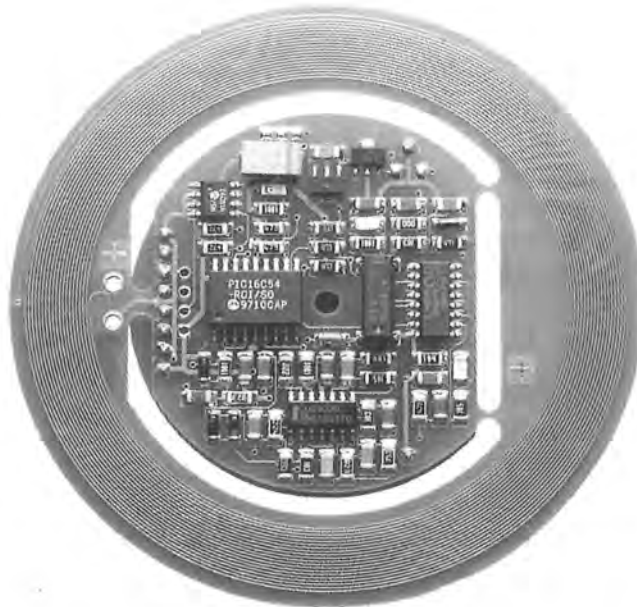
Figure 3.15 Reader for inductively coupled transponder in the frequency range < 135 kHz with integral antenna (reproduced by permission of easy-key System, micron, Halbergmoos)
