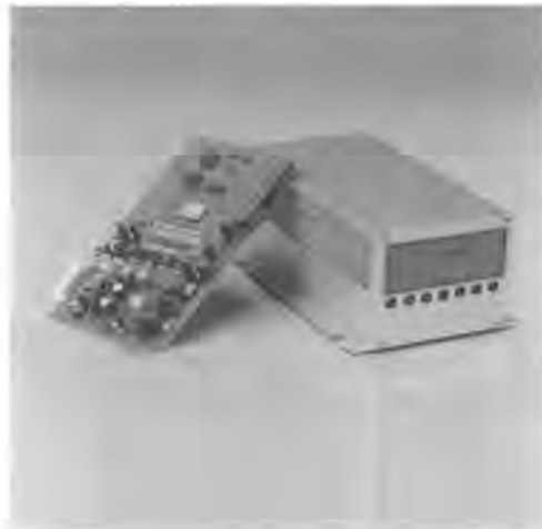
Figure 11.23 Example of an OEM reader for use in terminals or robots (photo: Long-Range/High-Speed Reader LHRI, reproduced by permission of SCEMTEC Transponder Technology GmbH, Reichshof-Wehrath)
