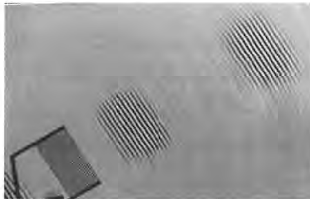
Figure 4.93 Scanning electron microscope photograph of several surface wave packets on a piezoelectric crystal. The interdigital transducer itself can be seen to the bottom left of the picture. An electric alternating voltage at the electrodes of the interdigital transducer generates a surface wave in the crystal lattice as a result of the piezoelectric effect. Conversely, an incoming surface wave generates an electric alternating voltage of the same frequency at the electrodes of the transducer (reproduced by permission of Siemens AG, ZT KM, Munich)
