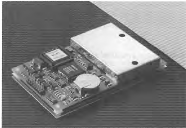
Figure 11.3 Example of a reader. The two functional blocks, HF interface and control system, can be clearly differentiated (MIFARE® reader, reproduced by permission of Philips Electronics N.V.)
