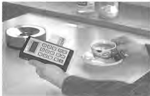
Figure 11.24 Reader for portable use in payment transactions or for service purposes. (Photo of LEGIC® reader reproduced by permission of Kaba Security Locking Systems AG, CH-Wetzikon)
