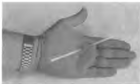
Figure 4.66 915 MHz transponder with a simple, extended dipole antenna. The transponder can be seen half way along (reproduced by permission of Trolleyscan, South Africa)
