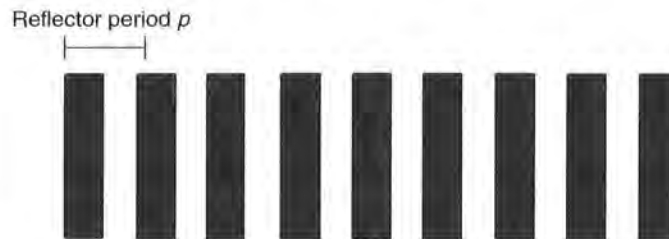
Figure 4.94 Geometry of a simple reflector for surface waves (reproduced by permission of Siemens AG, ZT KM, Munich)
