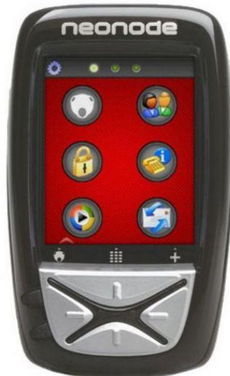
Figure 11: The first smartphone to support touch gestures: The Neonode N1 [Source: http://www.gsmhistory.com/vintage-mobiles/fig-36-neonode-n1/ ]
