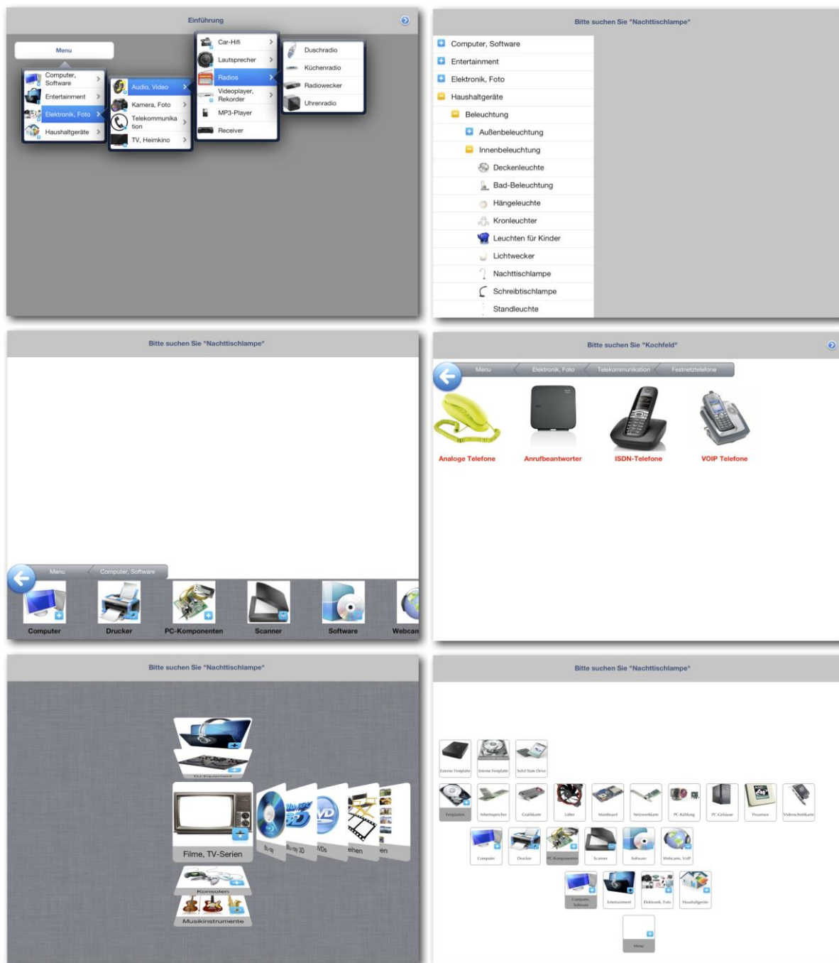
Figure 40: Six variants of novel menu concepts for touchscreen interaction, clockwise from top left: cascading dropdown, unfolding list, grid, tree, Cover Flow, and horizontal list [Source: Šahinagić et al., 2013]
