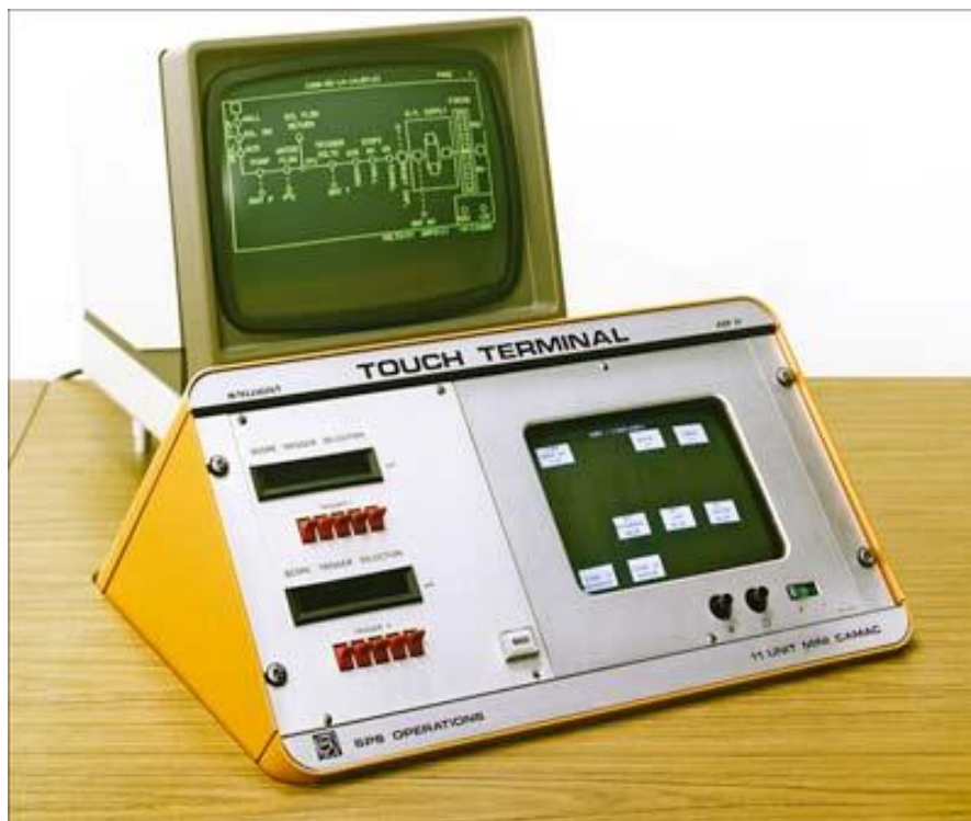
Figure 5: The first transparent, capacitive touchscreens (bottom) were developed and used at CERN. [Source: https://cerncourier.com/the-first-capacitive-touch-screens-at-cern/ ]
