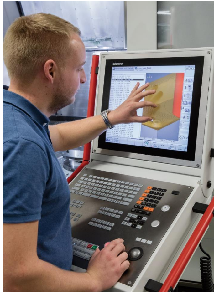
Figure 21: An engineer controls an industrial touchscreen system that supports direct manipulation via touch gestures. Nevertheless, the system offers a full keyboard, numerous function keys, and a trackball besides the touchscreen functionality. [Source: heidenhain.de]
