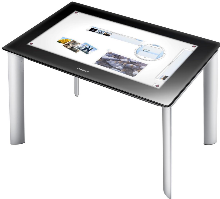
Figure 13: Touchscreen tables like the Samsung SUR40 allow multi-touch gesture interaction and can recognize objects that lie on the surface. [Source: http://nsquaredblog.blogspot.com/2012/07/australian-launch-event-for-samsung.html ]
