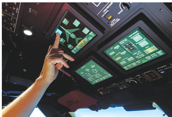
Figure 24: Due to easy integration, touchscreens will be integrated in a variety of places. This can lead to solutions that even require regular overhead use like this cockpit of a Gulfstream G500/G600. [Source: https://coeaerospace.com/cockpit-controls/ ]
