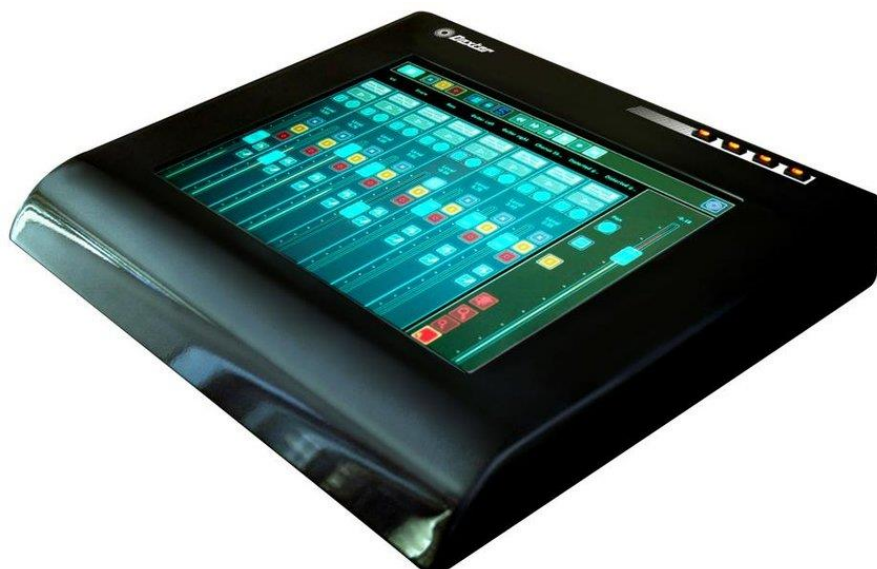
Figure 12: The Lemur music controller was the first commercially available touchscreen device that supported unlimited multi-touch. [Source: http://www.jazzmutant.com/ ]
