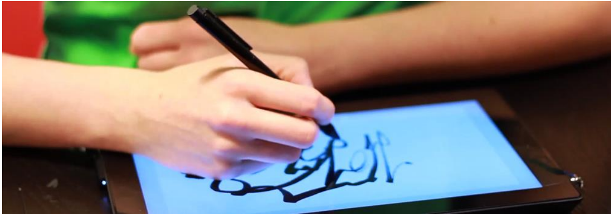
Figure 22: Palm recognition, also known as palm rejection, allows users to rest their hands on a horizontal touchscreen in an attempt to reduce strain on the arms and improve input precision. It is mostly integrated in touchscreen systems that can be controlled with a stylus. [Source: https://www.robertxiao.ca/research/ ]
