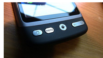
Frontal buttons (home, menu/options, go back, search) and optical track pad of an HTC Desire , a 2010 smartphone with Android OS .
