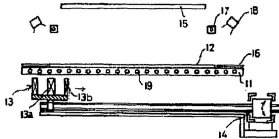
**ABSTRACT :** **PURPOSE** To provide the magnetron sputtering device which improves the efficiency of using a target and can prevent the generation of impurities by sputtering, etc.
