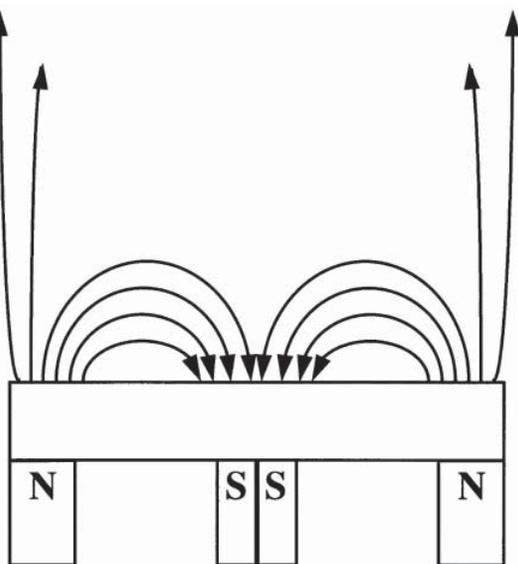
**Figure 2.** Schematic drawing of an unbalanced magnetron sputtering cathode.
