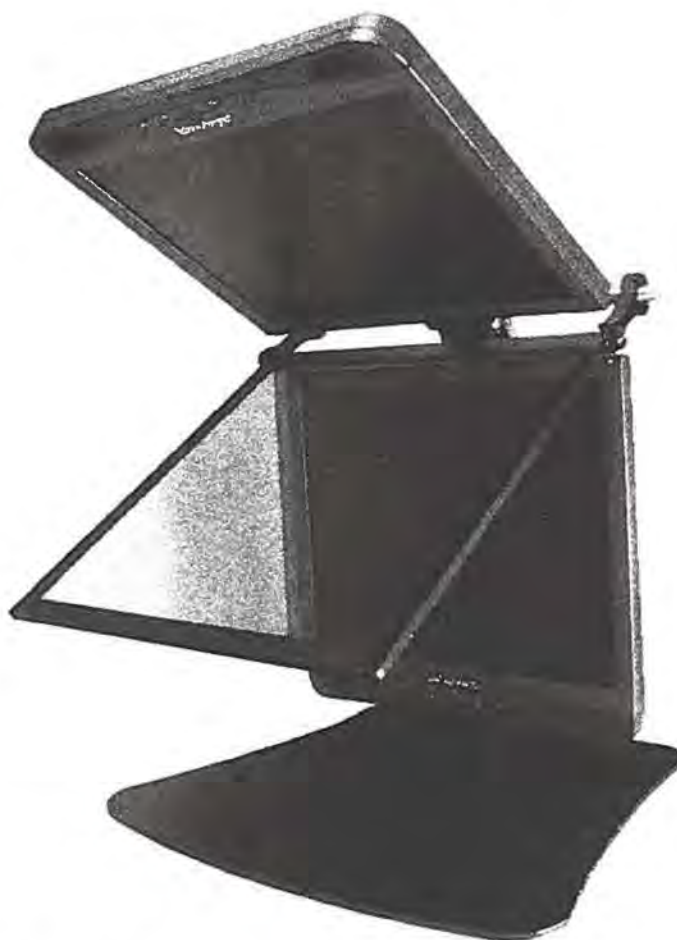
Figure 7.10: Stereomirror™ display using two AMLCDs and a half mirror, marketed by Planar Systems, Inc. [2].
