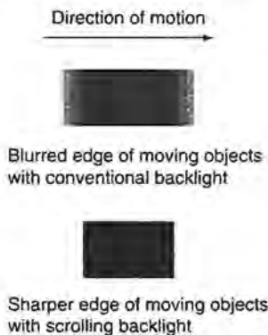
Figure 6.36: Qualitative improvement in motion portrayal with impulse-type (scanning or scrolling) backlight.
