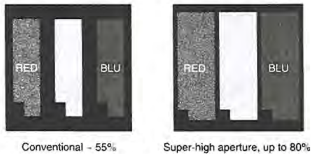
Figure 6.4: Comparison of aperture ratios in conventional and super-high-aperture ratio pixel designs as observed on a close-up view of an AMLC.
