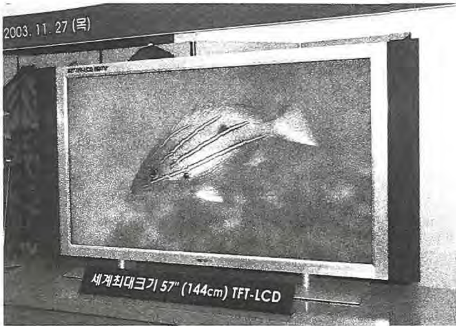
Figure 6.40: Photograph of a 57-in. TFT LCD developed by Samsung Electronics.
