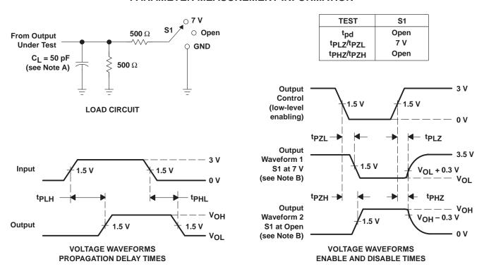
NOTES: A.  $C_L$  includes probe and jig capacitance.
