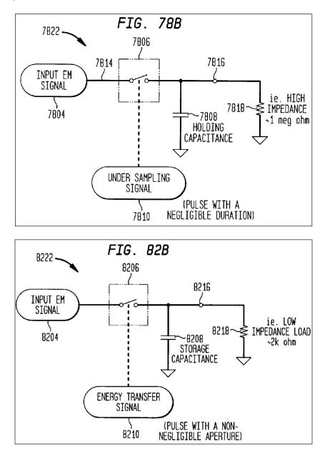
While Figures 78B and 82B depict that the respective circuits have a similar structure, their respective parameter values (*e.g.*, capacitor and load impedance values)—and concomitantly their respective operation—are very different. It is important to note that the input signal, input EM signal, is the same in both figures.
