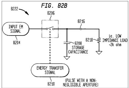
While Figures 78B and 82B depict that the respective circuits have a similar structure, their respective parameter values (*e.g.*, capacitor and load impedance values)—and concomitantly their respective operation—are very different. It is important to note that the input signal, input EM signal, is the same in both figures.
