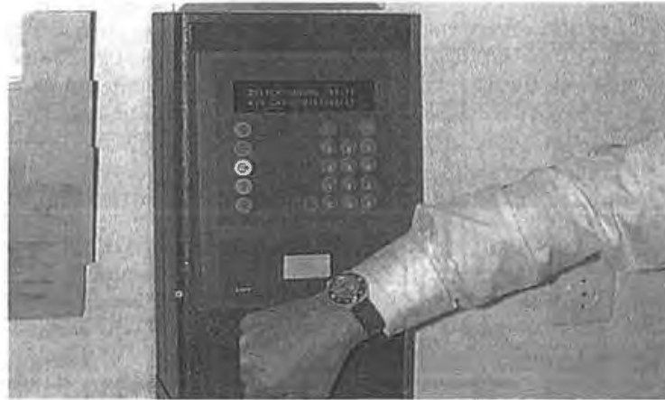
Figure 13.14: Access control and time keeping are combined in a single terminal. The clock with an integral transponder performs the function of a contactless data carrier. (Reproduced by permission of Legic Identsystems, CH-Wetzikon)
