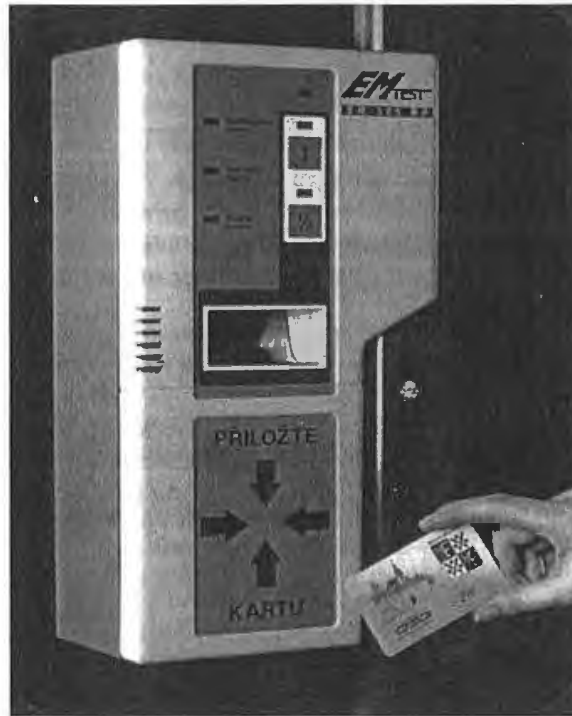
Figure 13.3: Contactless reader in a public transport system. (Photo: Frydek-Mistek project, Czechoslovakia, source: Reproduced by permission of EM Test)
