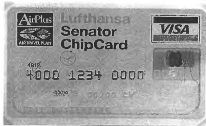
Figure 13.10: Miles & More – Senator ChipCard, partially cut away. The transponder module and antenna are clearly visible at the right-hand edge of the picture underneath the hologram. (Reproduced by permission of Giesecke & Devrient, Munich)
