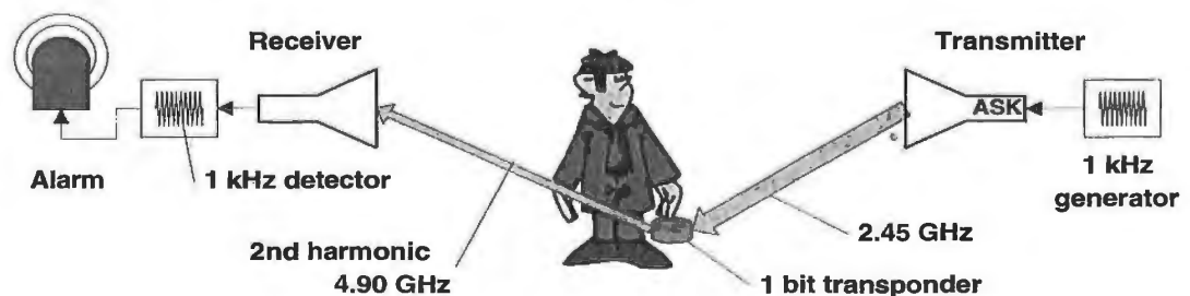
Figure 3.6: Microwave tag in the interrogation zone of a detector
