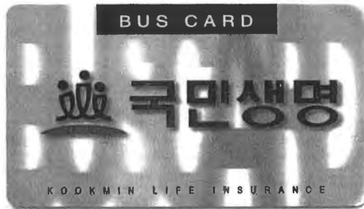
Figure 13.6: Contactless smart card for paying for journeys in a scheduled bus in Seoul (Reproduced by permission of Klaus Finkenzeller, Munich)
