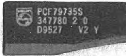
Figure 2.4: Transponder in a plastic housing. (Reproduced by permission of Philips Electronics B.V.)
