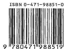
Figure 1.3: This barcode is printed on the back of this book and contains the ISBN number of the book.
