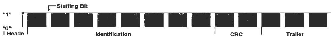
Figure 9.3: Structure of the load modulation data telegram comprising of starting sequence (header), ID code and check sum and trailer
