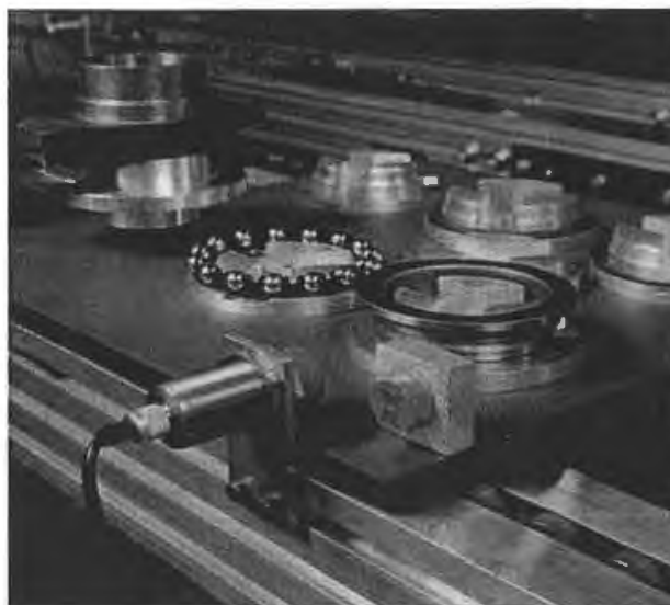
Figure 13.46: Individual components of a clutch release stop on a revolving pallet. Transponder and reader antenna are visible in the lower part of the photo (Reproduced by permission of Pepperl & Fuchs, Mannheim)
