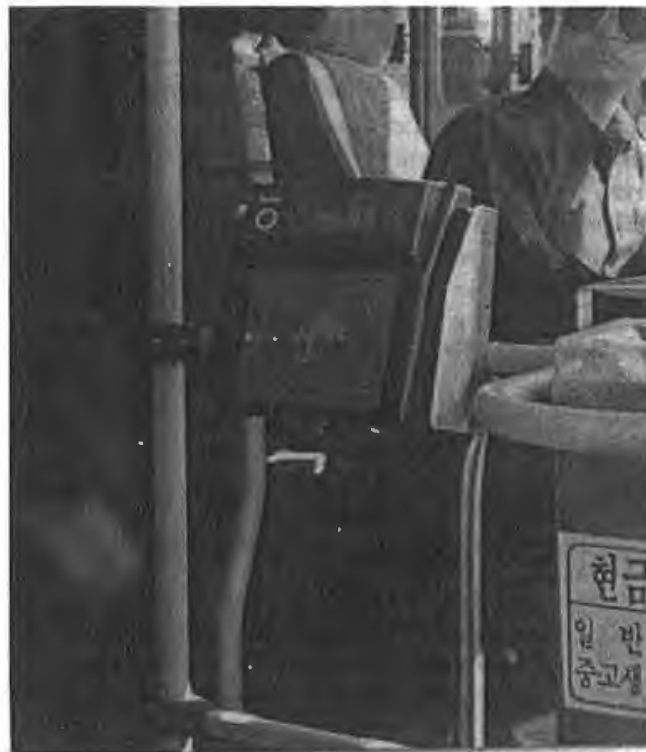
Figure 13.7: Reader for contactless smart cards at the entrance of a scheduled bus in Seoul (Reproduced by permission of Klaus Finkenzeller, Munich)
