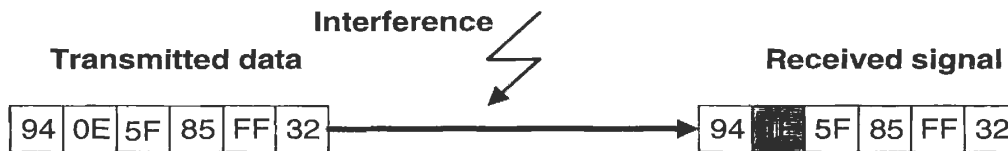
Figure 7.1: Interference during transmission can lead to errors in the data
