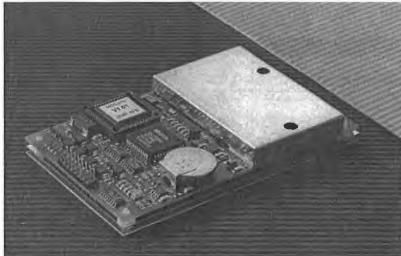
Figure 11.3: Example of a reader. The two functional blocks, HF interface and control system, can be clearly differentiated. (MIFARE® reader, reproduced by permission of Philips Electronics N.V.)
