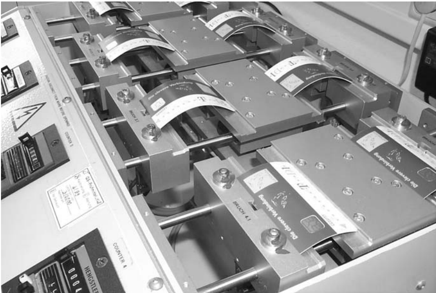
Figure 9.4 A machine for conducting dynamic bending tests on smart cards
