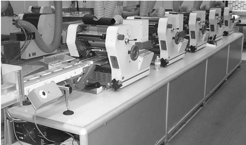
Figure 10.28 Five single-card silkscreen printing machines arranged in series
