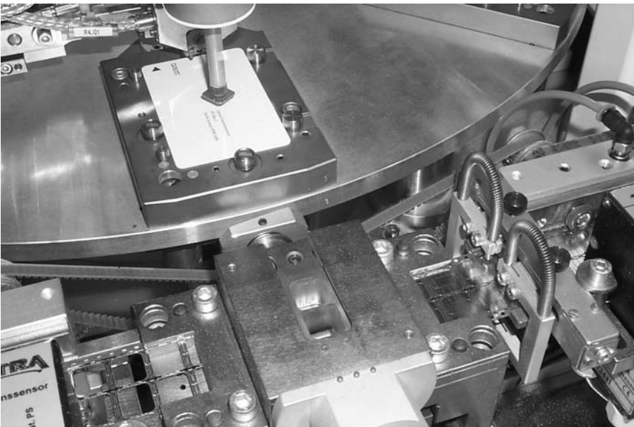
Figure 10.46 A rotary-table machine for implanting chip modules. The modules, which are arranged in pairs on the 35-mm carrier tape, can be seen in the foreground together with a small punch, from which they are lifted by a suction device and placed in the cavity of the card body
