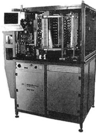
Figure 10.57 An initialization machine that can process 40 cards in parallel ( Source: Mühlbauer )
