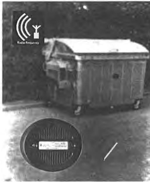
Figure 13.34: Dustbin transponder for fitting onto metal surfaces. (Reproduced by permission of Deister Electronic, Barsinghausen)
