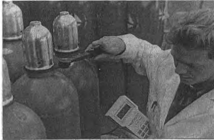
Figure 13.32: Identification of gas bottles using a portable reader. The reader (scemtec SIH3) is designed to function with transponders from different manufacturers. (Reproduced by permission of Messer Griesheim)
