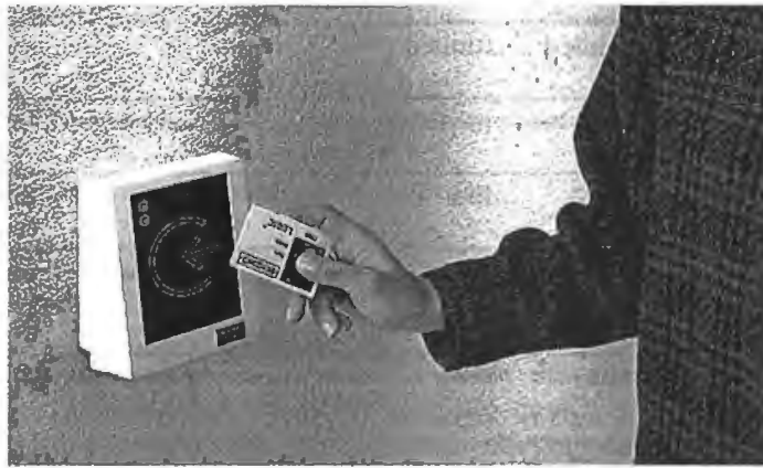
Figure 1.7: RFID reader and contactless smart card in practical use. (Reproduced by permission of Kaba Legic)
