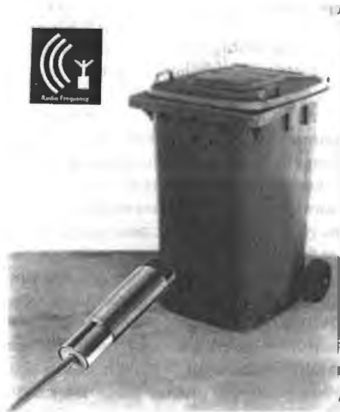
Figure 13.35: Reader antenna for installation in the dustcart. A plastic dustbin fitted with a transponder is shown in the background. (Reproduced by permission of Deister Electronic, Barsinghausen)
