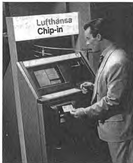
Figure 13.11: Passenger checking in using the contactless Miles & More Frequent Flyer Card. (Reproduced by permission of Lufthansa)
