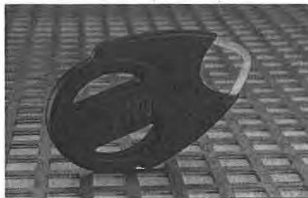
Figure 2.8: Keyring transponder for an access system (Reproduced by permission of Intermarketing)
