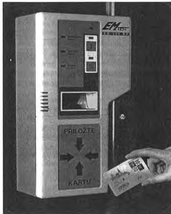
Figure 13.3: Contactless reader in a public transport system. (Photo: Frydek-Mistek project, Czechoslovakia, source: Reproduced by permission of EM Test)
