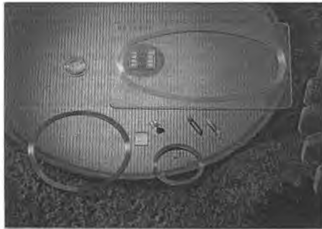
Figure 3.11: Different designs of inductively coupled transponders. The photo shows half finished transponders, i.e. transponders before injection into a plastic housing (Reproduced by permission of AmaTech GmbH & Co. KG, D-Pfronten)
