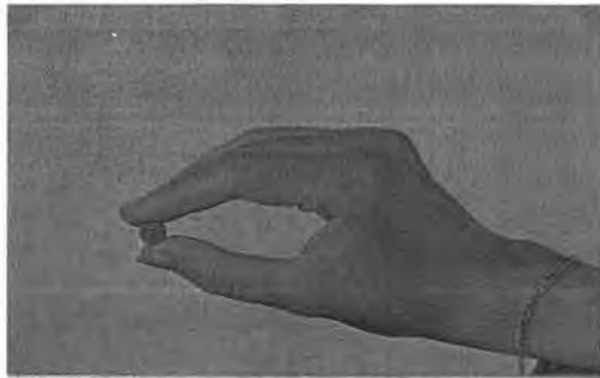
Figure 2.6: Transponder in a standardised construction format in accordance with ISO 69873, for fitting into one of the retention knobs of a CNC tool. (Reproduced by permission of Leitz GmbH & Co, Oberkochen)
