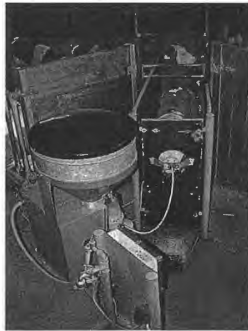
Figure 13.26: Example of automated animal recognition in practice: Grouping calves properly for feeding often requires much time and effort. Here a machine takes on this task: The animals can receive an individually adjustable amount of milk in several small portions. (Reproduced by permission of Dr. Michael Klindtworth, Bayerische Landesanstalt für Landtechnik, Freising)
