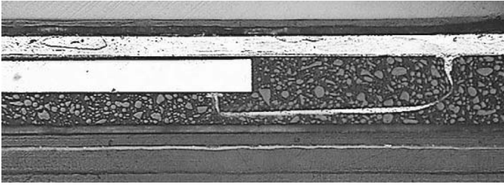
Figure 10.34 Detail of the cross-section of a chip module for contactless smart cards embedded in a card body. The bonding wire connecting the chip to the coil can be clearly seen ( Source: Giesecke & Devrient )
