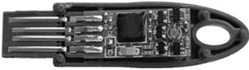
Figure 3.7 Example of a smart card with a different form factor. This photo shows a USB plug with a soldered-in smart card microcontroller and the necessary interface components, which has been opened up to reveal its internal components
