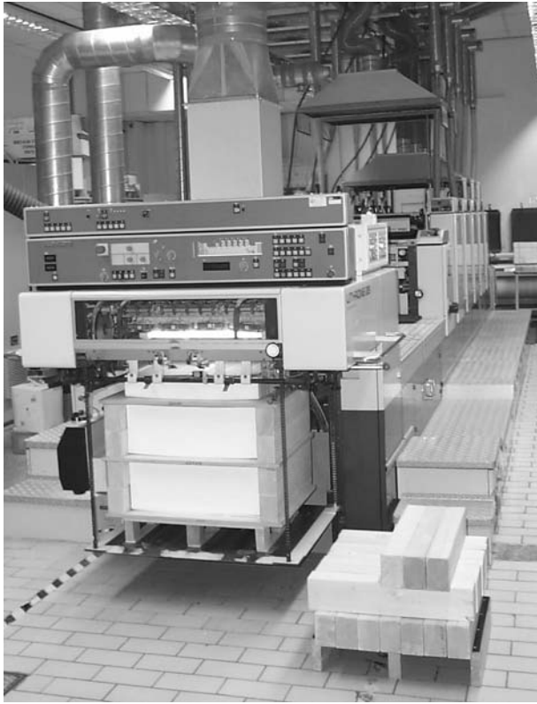
Figure 10.25 An offset printing machine for sheet printing
