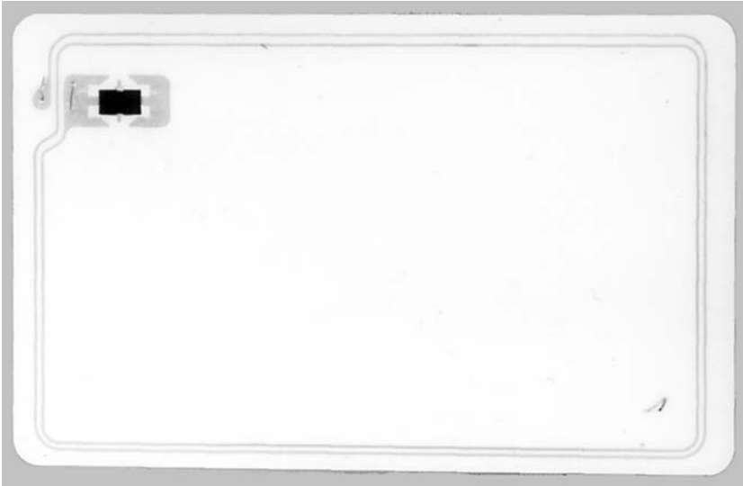
Figure 10.43 Printed coil for a contactless smart card
