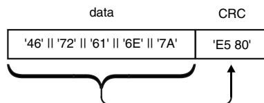
Figure 4.15 Sample computation of a CRC checksum using the generator polynomial G(x) = x^{16} + x^{12} + x^5 + 1 and an initial value of '0000'
