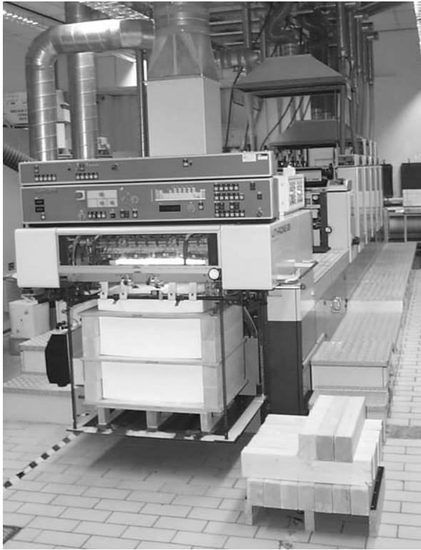
Figure 10.25 An offset printing machine for sheet printing
