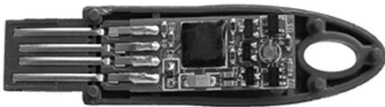
Figure 3.7 Example of a smart card with a different form factor. This photo shows a USB plug with a soldered-in smart card microcontroller and the necessary interface components, which has been opened up to reveal its internal components
