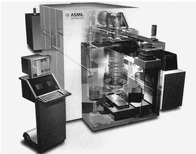
Figure 10.9 Cross-sectional drawing of a stepper for the stepwise optical exposure of individual semiconductor chips (Source: ASM Lithography)
