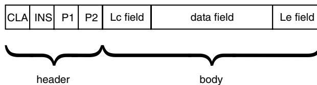
Figure 6.39 Structure of a command APDU
